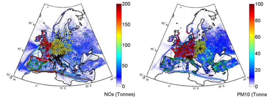
NO<sub>x</sub> and PM10 measurement stations overlaid over corresponding emission maps. Symbols colored according to evaluation subdomain.
