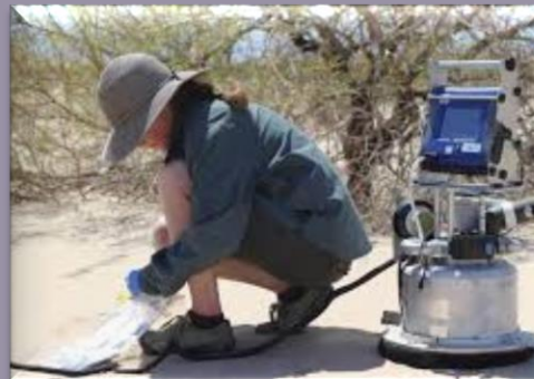
Figure 4. Karen Foley collecting samples in the Mojave Desert and a wind shear chamber device used for measuring landscape dust emission potential.
