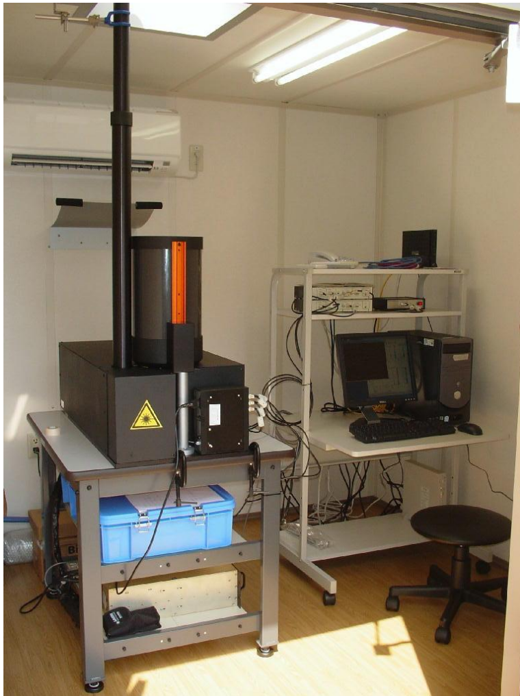
Two-wavelength (1064nm, 532nm) Mie-scattering lidar with polarization channels at 532nm. (Raman receivers (607nm) are being added at several observation sites.)
