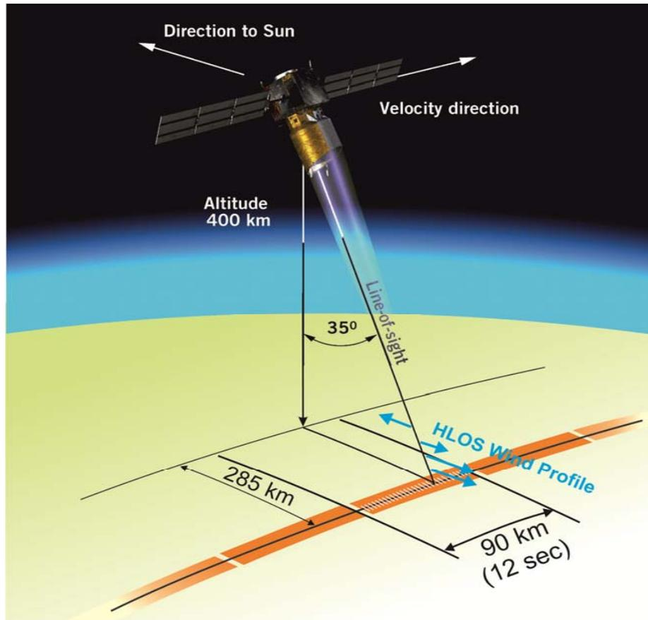
UV lidar (355 nm , circularly polarized)
