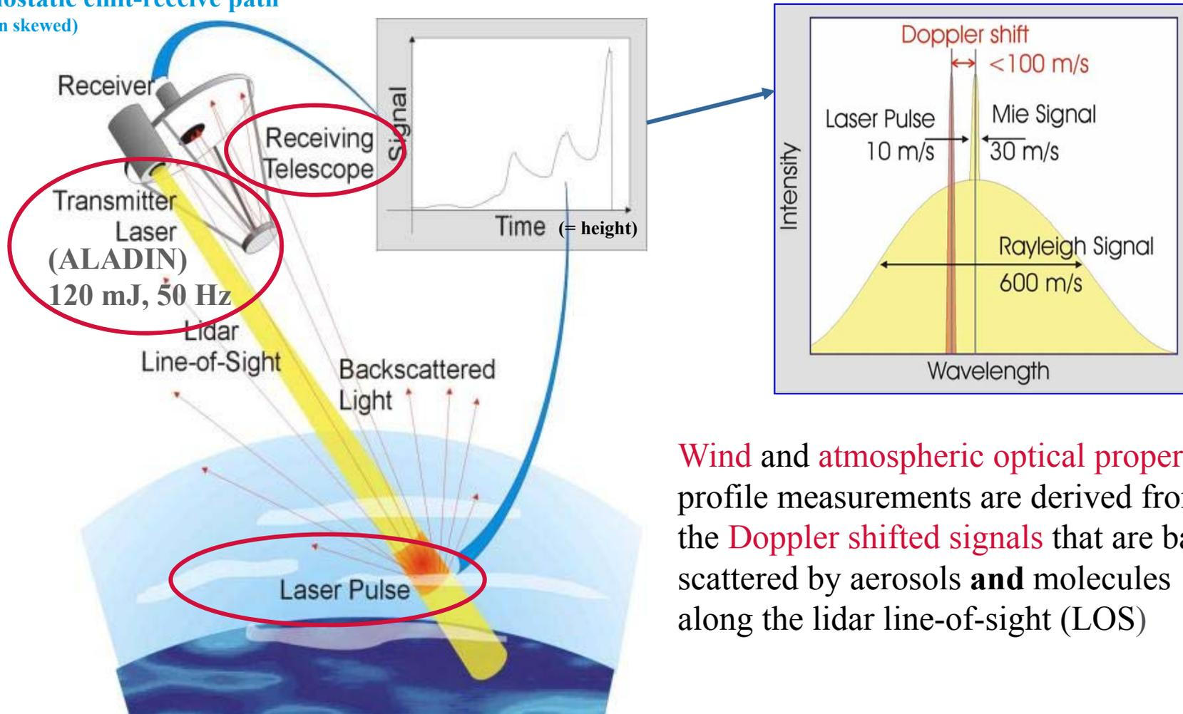
Wind and atmospheric optical properties profile measurements are derived from the Doppler shifted signals that are back-scattered by aerosols **and** molecules along the lidar line-of-sight (LOS)
