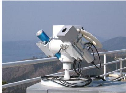
**Precision Filter Radiometer
