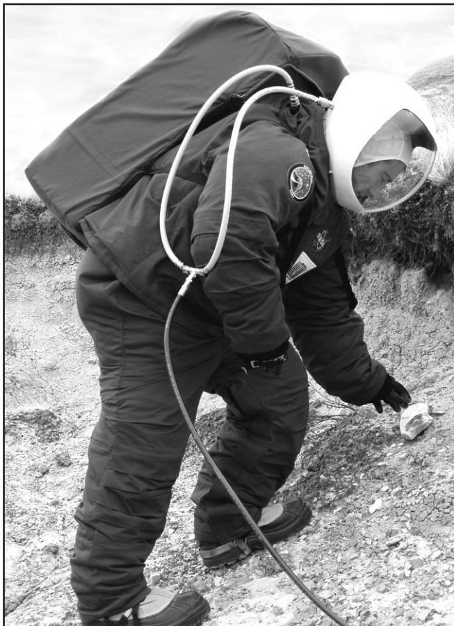
The NDX-1 Space Suit was tested for five days in the Mars-like terrain of the North Dakota Badlands. A four-minute videotape of the test can be accessed at www.space.edu/spacegrant/research.html .
