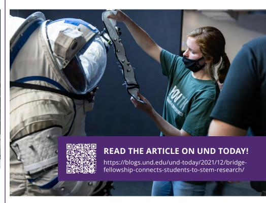
Liz Deckert checks the placement of reflective balls that sit atop a Velcro strap before attaching the strap to the arm of her volunteer. The balls bounce infrared light back to 18 different cameras, which can triangulate marker positions in 3D space. Once researchers have a clean marker set, they can run the video through sophisticated software to collect detailed kinetic data. Photo by Mike Hess/UND Today
