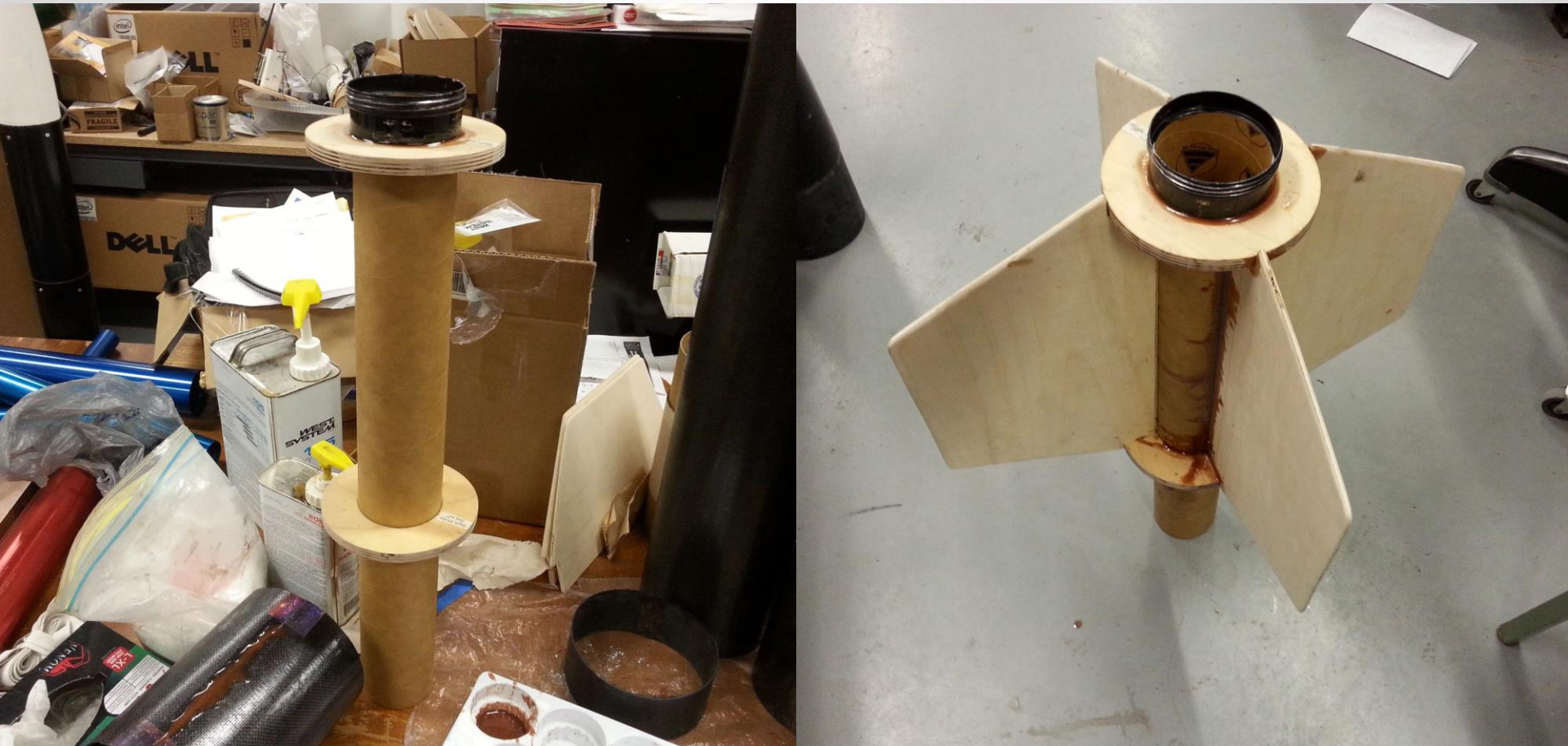
Fin Can and Motor Mount
