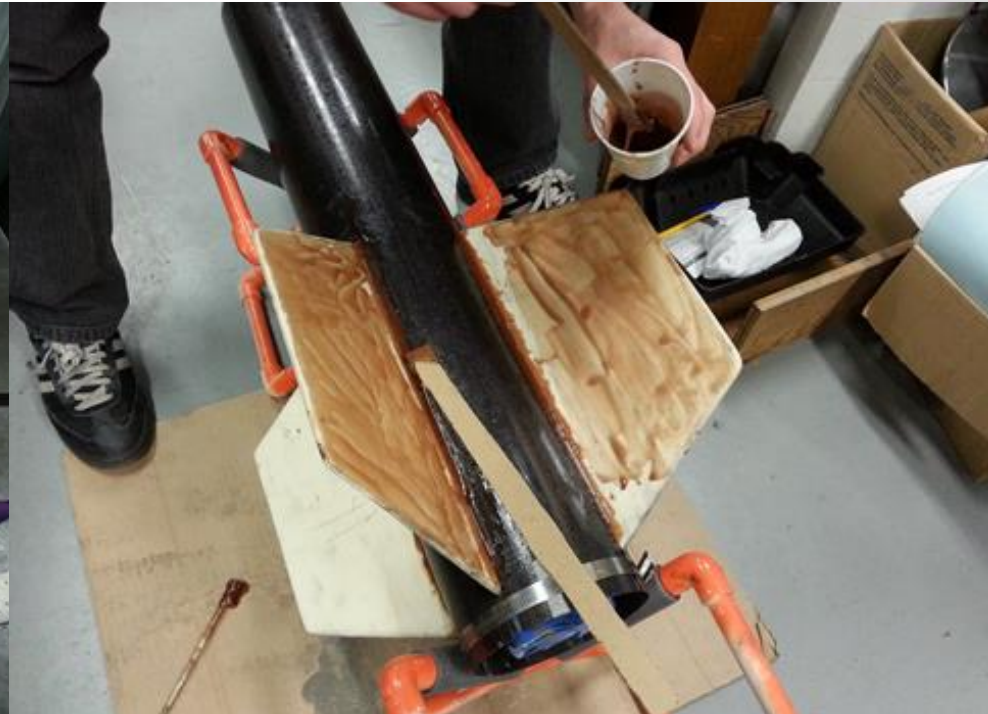
Epoxying of the fins
