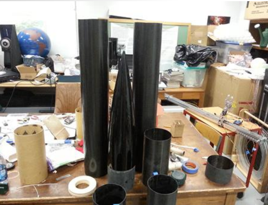
Carbon fiber tubes reception from China (after cutting)
