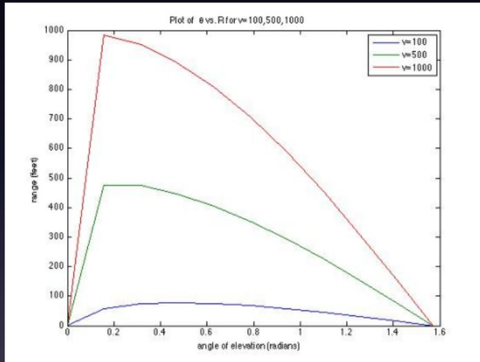
Figure : Plot of theta vs. range for varying values of speed:  $v=100, 500, 1000$  and  $k=1$
