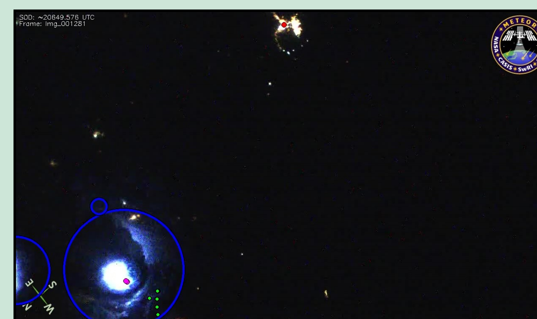
Final output of algorithm. The blue circles represent the minimum bounding circles around contours meeting a minimum radius of ten pixels. The green dots represent ISS-LIS event data, whereas the fuchsia dots are NLDN flash data. The single red dot is Del Rio, TX. Note the offset between ISS-LIS and NLDN Data.
