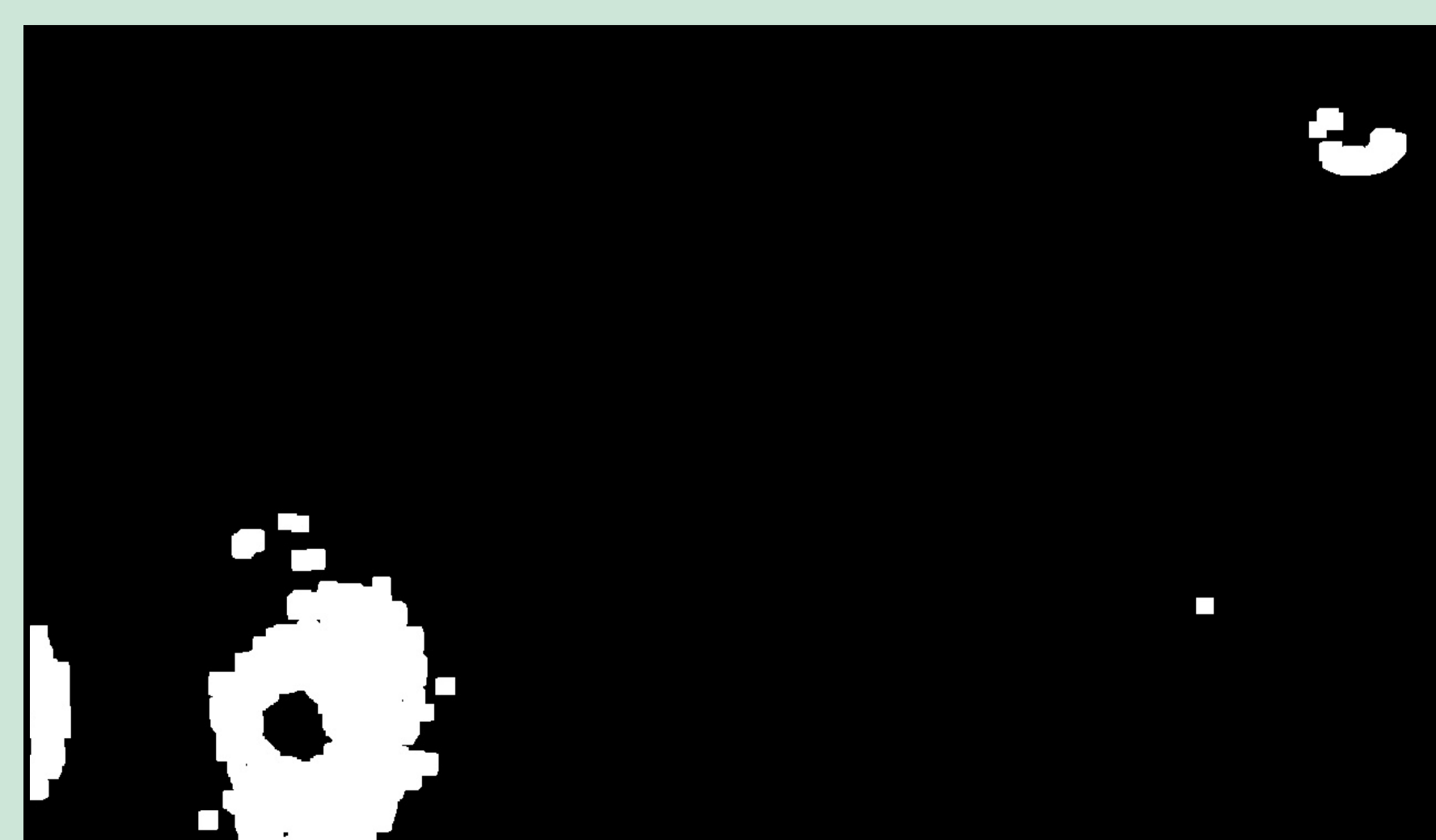
Red Green Chromaticity image after conversion to Hue Saturation Value color space and application of thresholds to find pixels with highest blue values. The resulting image is a binary mask that has undergone one erosion and seven dilations in order to remove high frequency noise and combine fragmented contours.
