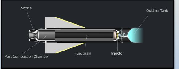
Goal: Design and Characterize a PMMA/GOx based hybrid rocket propulsion system. We want to investigate the combustion behavior, fuel regression and propulsion of the engine design.
