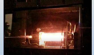
Void entrainment was observed by the acrylic fuel grain, and more importantly the fuel core survived the test showing success of the design.
