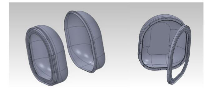
Left: Suitport assembly that connects to the NDX-2. Right: Rover mount and suitport dock. Spacesuit portion of suitport in open configuration for donning/doffing.
