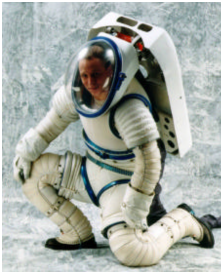
Figure-12 ILC Dover's "T" Suit. Note Oval Helmet
